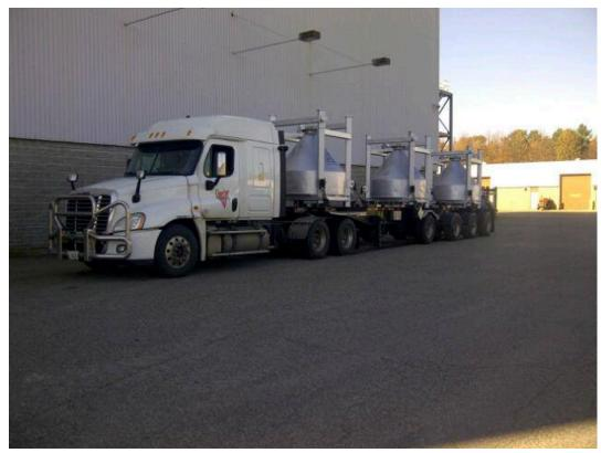
Figure 3-2: Shipping totes used to transfer UO<sub>3</sub> from Blind River Refinery to the Port Hope Conversion Facility
